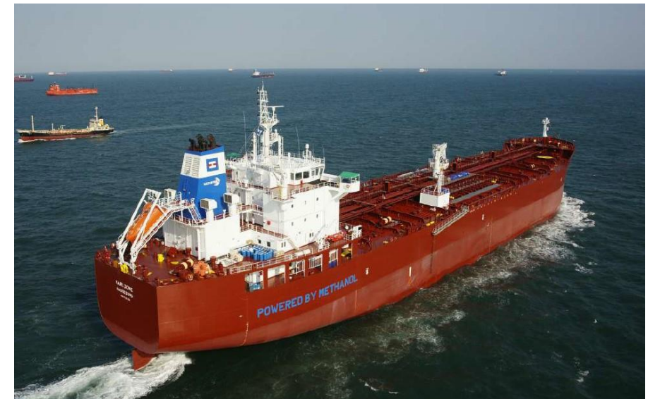
Ocean-going vessel powered by methanol
