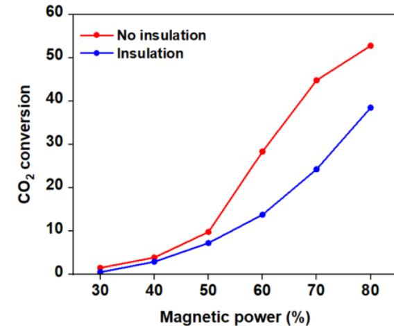
**Addition of simple heating jacket improves conversion by up to 14%**
