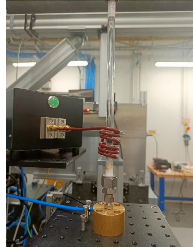
Increasing magnetic field strength during CO<sub>2</sub> conversion.
